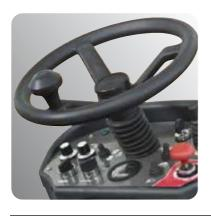
Control panel with easy and intuitive controls featuring: hour meter, battery charge level indicator, empty tank light and forward/reverse drive indicator. Speed adjustment, horn, main brush pressure adjustment,
